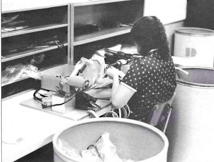
Attaching the grip to the racquet.
