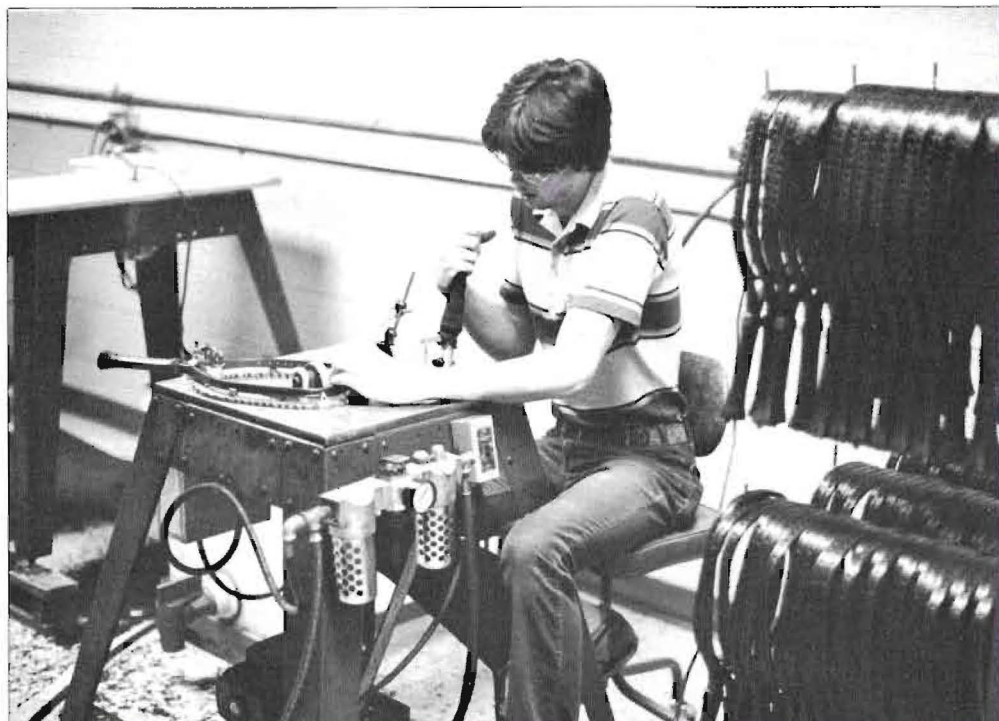
Hand-drilling an injection molded racquet.
