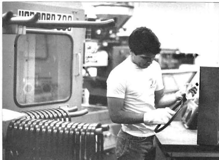
Molding racquet frames in the Richcraft factory.
