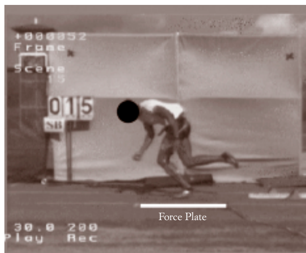
Figure 2. Sprint start performed from blocks positioned just in front of force-plate installed within the track. Force plate was used to measure ground reaction forces generated during the first step out of the starting blocks.
