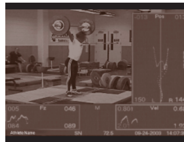
Figure 2. Display of synchronized video and measured variables during one moment in time at the end of the lifting motion.
